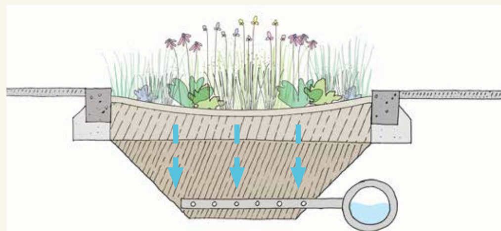
Above: water permeating through the rain garden is taken away via a perforated pipe. Sometimes referred to as a lined system.
